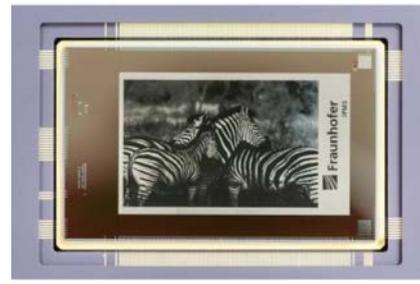
Figure 1: Ceramic-packaged 48 $\mu$ m, 512 x 320 Tip-Tilt micro mirror array with a programmed pattern (right) [2].
