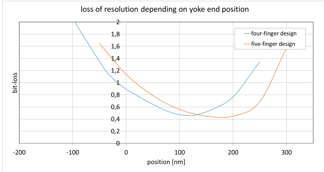
Figure 7: comparison of the actuator behavior depending on the linearity
