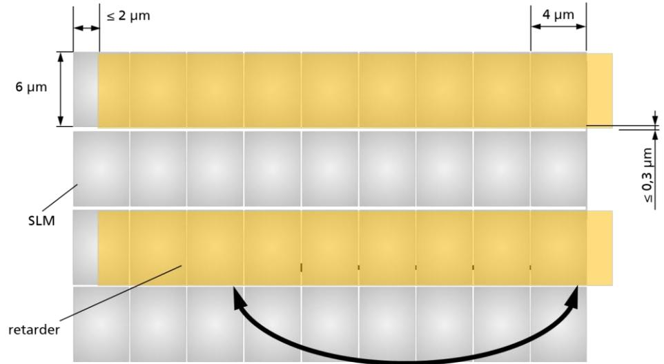
Angular alignment needs to comply with the linear  $\leq 0,3 \mu\text{m}$  criteria
