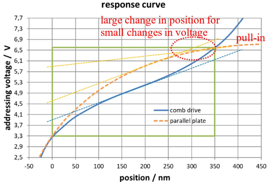
the parallel plate actuator needs to have a much weaker hinge than the comb drive actuator for the same deflection
