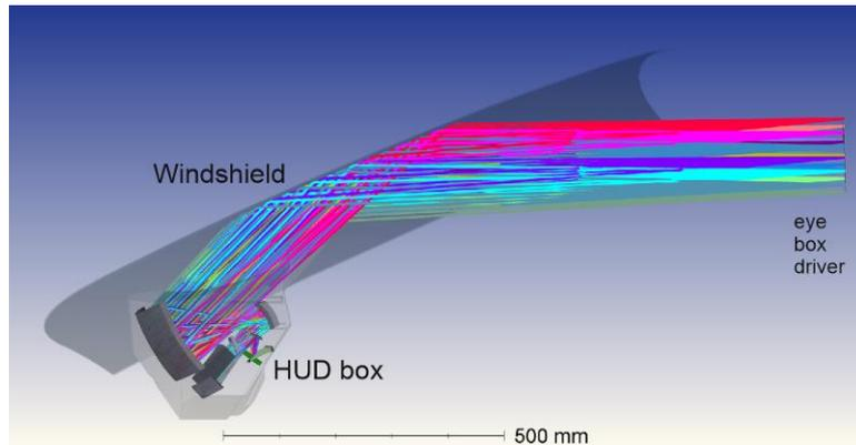
Figure 3. Example of a Zemax optical design of a holographic HUD. This design is more compact than the current experimental implementation and shows the potential of future integration of the HUD into a car. The lab-setup already uses a similar arrangement of components but the size and distance of some parts is still larger.
