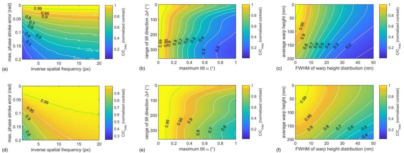
Figure 10. Comparative analysis of simulated reconstruction quality represented by the dependency of the normalized background contrast on various potential mirror errors (phase stroke, tilt, and warp) for both Fresnel (top) and Fourier (bottom) holograms.
