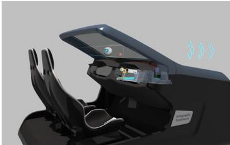
Figure 1. Schematic view of HUD set-up at SeeReal. The driver can see objects at different distances in front of or even inside the car, that are generated by a holographic HUD. Photos in the following figures are made with a camera located at the position of the driver's head.
