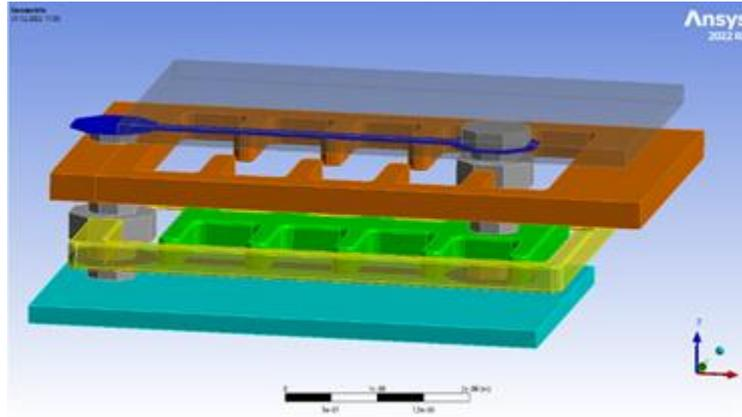
Figure 9. Mechanical design of single mirror with 4x6 micron pitch with fixed stator plate (orange), dual springs (blue) and moveable yoke (green).
