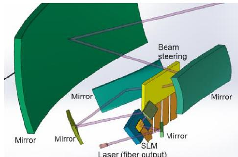
Figure 4. Details of the HUD design: components in the HUD box.
