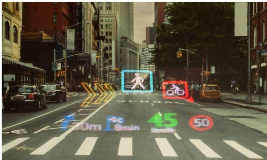
Figure 2. Street scene with HUD symbols and camera focus either on front or back (real holographic reconstruction – photos taken by camera, but in an indoor environment, not on a real street).
