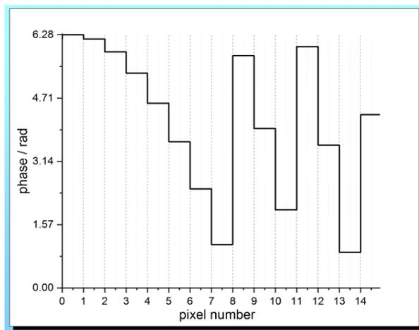
Figure 6. Right half of a Sub-hologram lens function – similar to a Fresnel lens.
