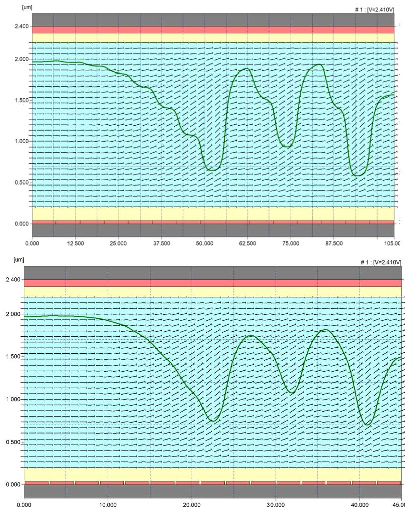
Figure 7. Liquid crystal simulation for an LCOS with a pixel pitch of 7  $\mu\text{m}$  (upper part of the figure) or with a pitch of 3  $\mu\text{m}$  (lower part of the figure) respectively, showing half of a sub-hologram and the smoothing of the sub-hologram phase function due to fringe fields and LC response. The impact of smoothing is more pronounced for the smaller pitch.
