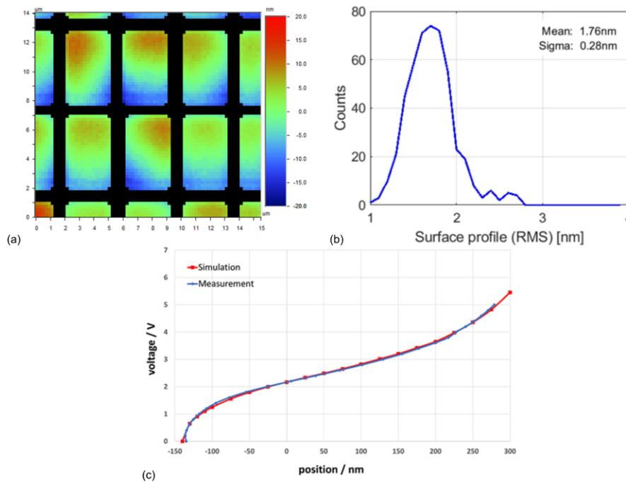
Figure 11. Optical assessment of mirror surfaces of a MEMS prototype. (a) Spatially resolved height profiles. (b) RMS histogram after numerical subtraction of plane tilt. (c) Voltage-Offset characteristic.
